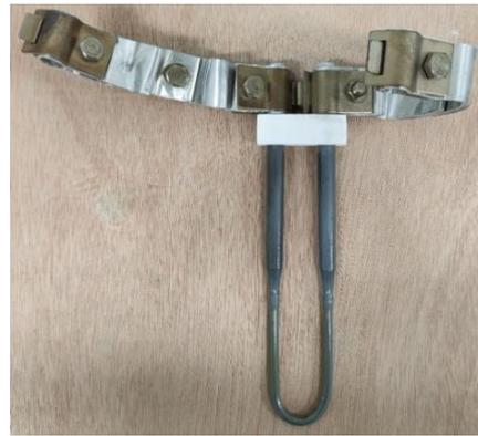
Step 4: Install the silicon-molybdenum rod with the connecting piece into the silicon-molybdenum rod holes in the chamber, and connect it in series with the neighboring silicon-molybdenum rods:
