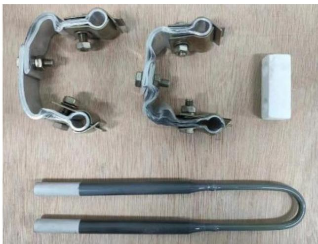
Step 2: Remove the wooden block in the middle of the silicon-molybdenum rod and pass the rod through the holes of the brick:
