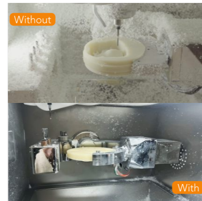
Integrated ionizer neutralizes the electrostatic charge of chips (PMMA/plastics)
