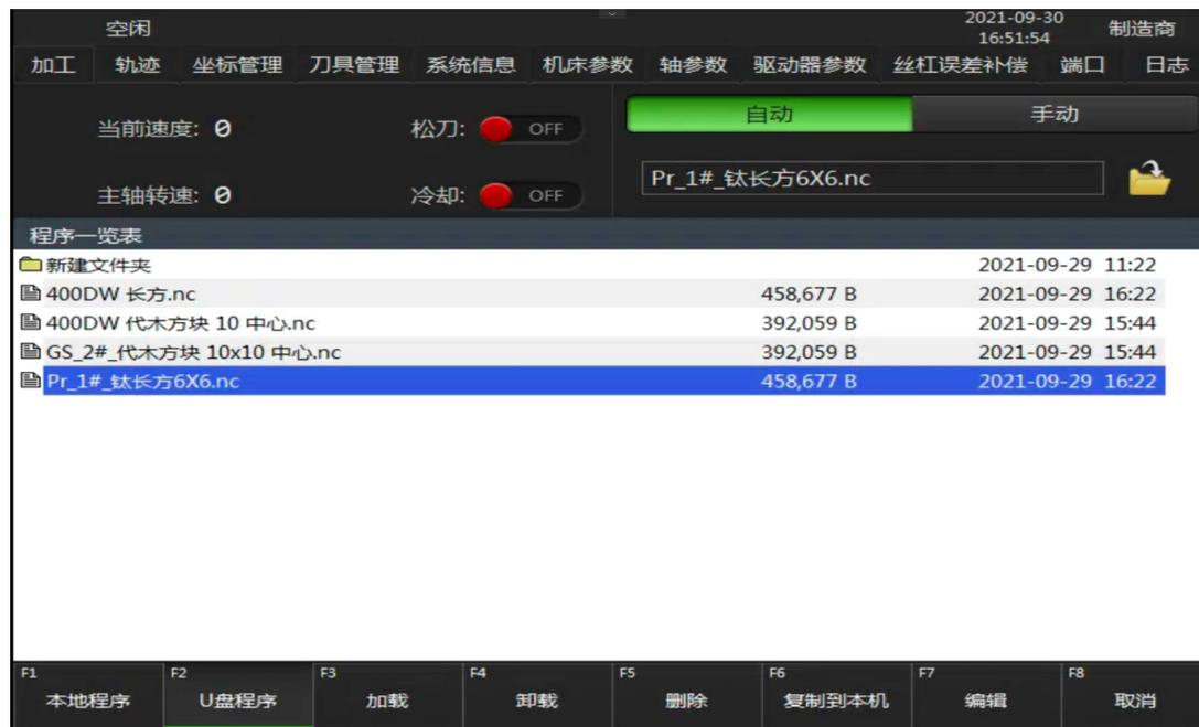
3) When a sentence "Processing program loading succeeded" shows on the machine operation interface, it means that the program you chosen is imported successfully and the file name of the imported program is displayed at 1
