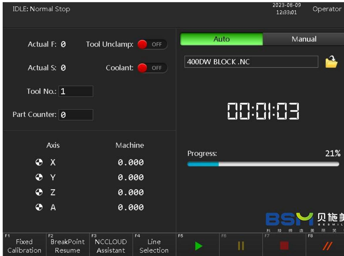
4) Click the operation button "F5" on the machine operation interface to process the current program
